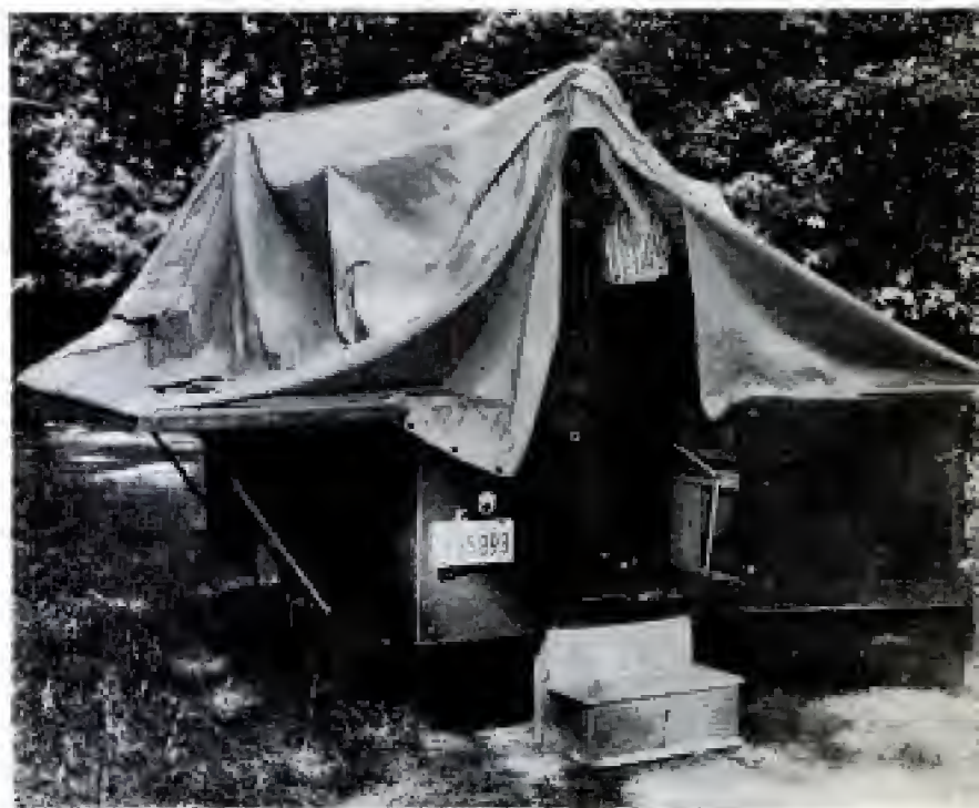
Above, pipe framework swings upward from trailer body to support tent roof like covered wagon. Steps under body keep trailer from tipping. Below, Jim Kendall buttons canvas to row of regular curtain fasteners which are added to front of trailer
